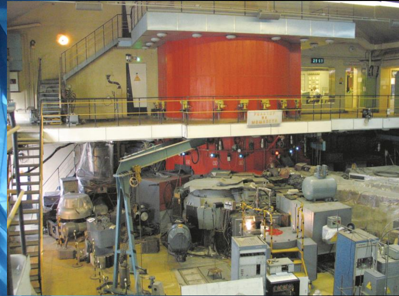
Source of thermal neutrons is a nuclear experimental reactor IR-8 in NRC KI with neutron flux of no less than 10^{12} \text{ cm}^{-2}\text{c}^{-1} ;
